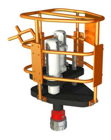
Simple in-situ setup, operation and retrieval by assistance of standard work class ROV The Stinger ROV Operated Drilling Tool is a portable hydraulically operated drilling machine which can be operated by a work class ROV. It is designed for subsea drilling operations on a variety of applications and steel thicknesses.
