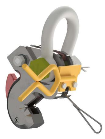
Designed for loads in parallel to normal direction relative to the riser The Imenco S-Hook Lifting Anchor is developed with a purpose to achieve a safe handling when steel structures e.g. riser pipes are being removed during demolition and decommissioning of offshore structures. The anchor is furthermore equipped with a self-locking latch dog that will automatically activate when the anchor is correctly mounted into a pre-drilled anchoring hole.
