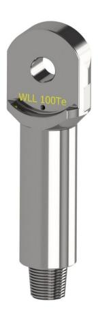
This unit connects the Running Tool to the lifting line for subsea installation and retrieval operations Imenco has developed and supplied dedicated 100Te WLL NC-50 Lifting Sub (NC-50 Lifting Adaptor/ Deployment Pup piece) for mounting on top of X-mas Tree Running Tool or other equipment. The sub has a cylindrical (box) area of sufficient length to enable make up and break out of the threaded connection using normal drill pipe rig tongs.
