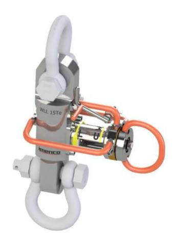
The combined weak link is a tool that combines Safe Lifting and Overload Protection in one ROV operated unit A 15Te Combined Weak Link is the perfect tool for easy and safe lifting while the lifting line has an ROV enabled overload protection available at all times. When in Weak Mode, an emergency release breaking point at a desired value is included in the lifting line. Switching between the two modes can be simply performed by work class ROV.
